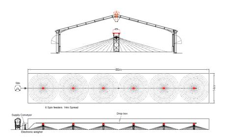
The design of the disk is a point of difference between manufacturers. Cheaper models have a simple disk that may provide quick and even distribution, but often gives a donut spin pattern, with the feed falling in a band around the feeder. More sophisticated designs spread the feed evenly underneath and around the feeder.
