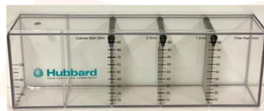
Figure 12: Hubbard Feed Sieve
